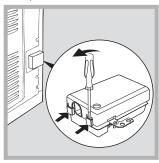
screwdriver into the side tabs of the cover. Use the screwdriver as a lever by pushing it down to open the cover (see diagram).
